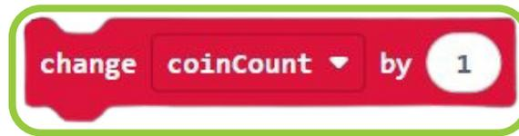
This block allows you to instruct the microcontroller to add a number to the number already in a variable.
