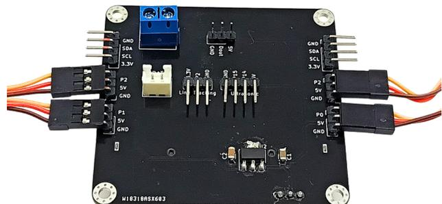
For the fourth servo, connect brown to Ground (GND), red to 5V, and yellow to P0. Then, turn your board around and press both black buttons simultaneously to calibrate the servos. Finally, remove all the servos.
