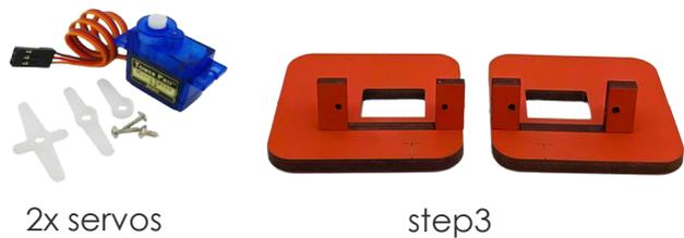
Place the servos on Board A1, ensuring that the shafts align with the "T" symbols on the board.
