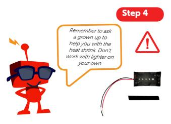
Refer to Step 1, the wiring diagram to connect the wires. First put the heat shrink tube on the black wire, connect the wire core to the boat switch, then completely cover the heat shrink tube, and shrink the heat shrink tube with a lighter to shrink it.
