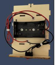
Use cable ties to organize the wires and trim off the excess cable tie with a scissor. Please be careful when arranging the wiring to avoid breaking the wires.
