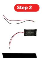
Refer to the circuit wiring diagram in Step 1, First put the heat shrink tube on the red wire and then connect the wire cores together, then completely cover the wire core with the heat shrink tube, bake the heat shrink tube with a lighter to make it shrink.
