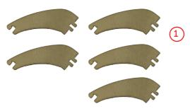
Continue adding board 1 - Just like in Step 1, add all board 1s onto the board 2.
