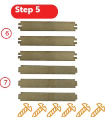
Install the three board 6s on the board 5 using three 4mm screws. You can do this in any order. Now, put the three board 7s on top of board 5.
