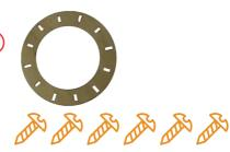
Use 6x 4mm screws to attach all board 1s to board 3. Remember to put them into the smaller holes of board 3.
