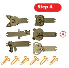
Attach all board 4s - Use 6x 4mm screws to fix all board 4s in place.
