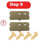
Install board 9 - Use 4x 4mm screws to attach the two board 9s separately onto board 8.
