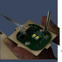
Press the black button on board 4, turn on the power, and cover the photoresistor on board 7 with your hand. If the LED light turns on, you're good to go. If not, use a small screwdriver to adjust the LED to the right until it lights up.
