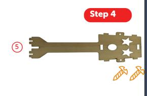
Install board 5 on top of boards 4 and 6 and secure it using 4mm screws.
