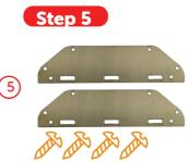
Attach two board 5s to board 3 using 7mm screws.
