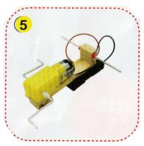
Step 5: Put the long shaft with bushings on each side through the vertical block. Add the angle shafts to the motor
