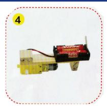
Step 4: Glue the motor on side of the vertical block and the battery holder on the side of the horizontal block (as shown)
