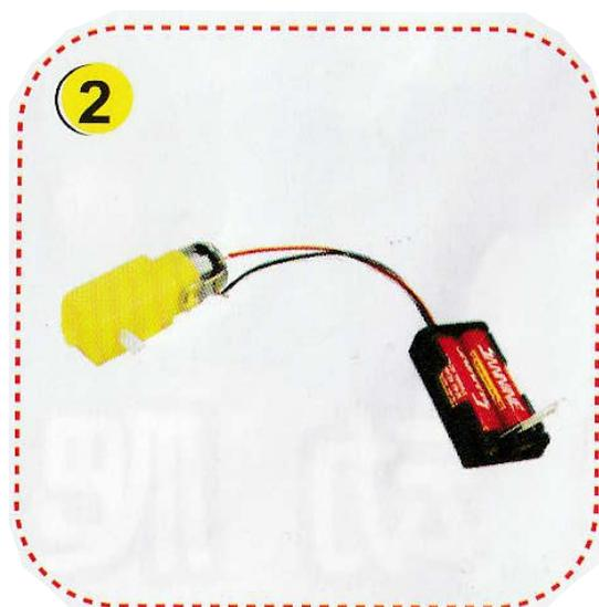
Step 2: Connect the wires to the motor. There is a small loop on each side where you can thread the wire through, twist the wire to secure
