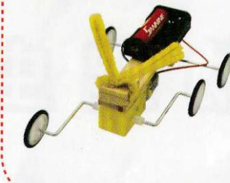
Step 8: Twist the pipe cleaner wire so you can add the eyes
