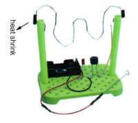
**Step 6:** Add heat shrink to the tips of the wire and fix the wires on the pillars
