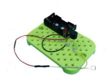
**Step 4:** Connect the wires of the battery holder to the buzzer and LED
