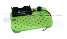
**Step 2:** Fasten the LED and the buzzer on the base plate make sure the + and - is correct
