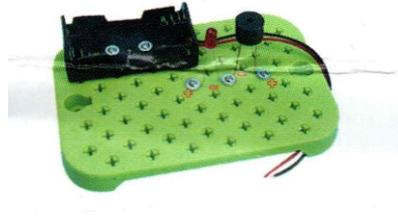
**Step 2:** Fasten the LED and the buzzer on the base plate
