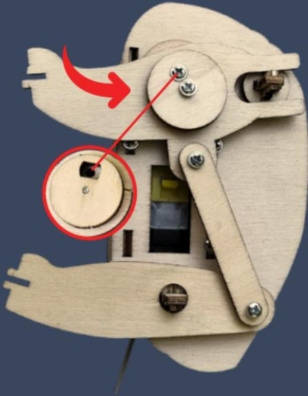
Time to bring those legs to life! Attach the legs to the wooden stakes and fix the “joints” onto the rotating shaft of the yellow motor using 7mm screws.
