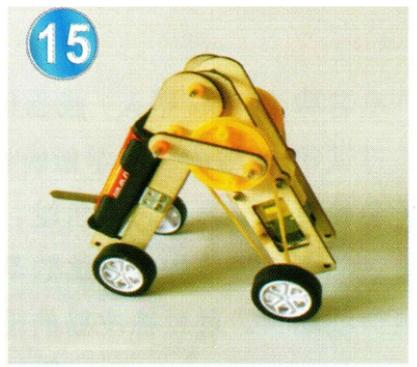
Step 15: Install two AA batteries and the production is complete.
