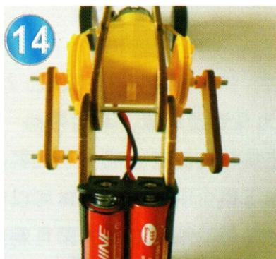
Step 14: Take part 6/7 and 4 bushings, divide into two bushings, and two rubber bands and install them as shown in the picture
