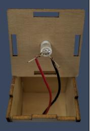
Put the LED into the fiber optic tube sleeve. Then, separate the LED parts (this prevents a short circuit).
