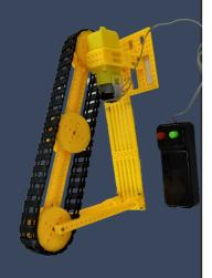
Next, we'll put tracks on the pulleys and slide the two 95mm plates into the base plates. Now, we'll slide the ends of the 40mm shaft through the two plates we just added. Finally, we'll connect the wires from the remote control to some copper plates on the yellow motor Incert the batteries and start Cody!
