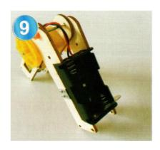
Step 9: Insert the battery box into the card slot of No. 1/2 piece, as shown in the figure. Note: If the battery box is not tight, add screws to fix it
