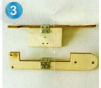
Step 3: Take the 3 piece and the angle iron, and fasten it with two small screw, as shown in the figure.
