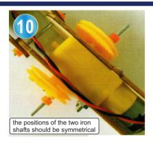
Step 10: Take 1.5cm long iron shaft and install them separately on the yellow wheel, install two bushings respectively, as the picture shows.
