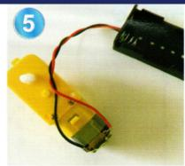
Step 5: Tighten the red and black wires of the battery box respectively on the two wiring contacts of the motor, as shown in the figure.
