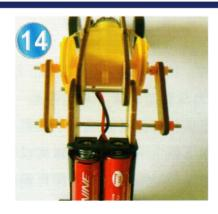
Step 14: Take part 6/7 and 4 bushings, divide into two bushings, and two rubber bands and install them as shown in the picture
