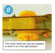
Step 8: Insert the two yellow wheels into the motor shaft respectively, and fix them with screws, as shown in the figure
