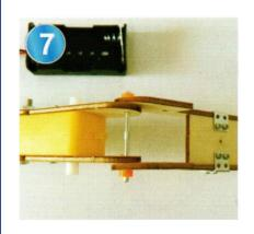
Step 7: Take a 4cm long iron shaft and two bushings, connect pieces 1-5, as shown in the figure
