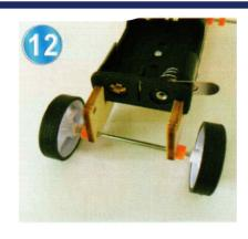
Step 12: Take 5 cm long iron shaft and two wheels. The sub is installed on the 1/2 piece. as the picture shows
