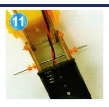
Step 11: Take 7 cm long iron shaft and 4 shaft sleeves Installed on the 1/2 piece, as shown in the picture
