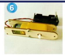
Step 6: Take the No. 4/5 part and fasten it with the motor with the screw nut, as shown in the figure.
